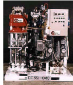
Covercat 351 A typical Plural Pump for EPFP
